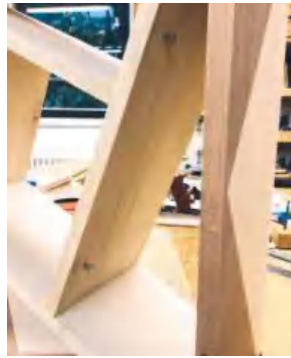
▲ Pic.39 As a stop, I used two little bolts on the open side of the drawer, which in this case, were on its side
